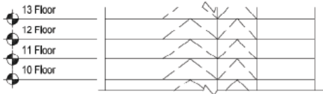
Figure 7: Typical Core E/W Core Bracing Elevation
